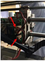
15 Slide the two RJ45 connectors into the RJ45 guard and then into the head PCB. When viewed from the front, the cable with the blue marking should go on the left, while the cable with the green marking goes on the right. Make sure they snap securely. The edge of the black RJ45 guard should slide 1-2mm over the side of the green PCB:
