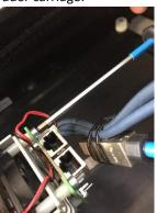
14 Identify the cooling block fan, and print cooling fan and their connectors. The print cooling fan is the radial fan connected to the fan duct close to the nozzle. Connect the cooling block fan to the top fan connector on the head PCB (the one marked 'head'). Connect the print cooling fan to the bottom fan connector on the head PCB:
