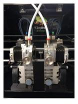
2 Disconnect the four RJ45 connectors from the left and right extruder heads:
