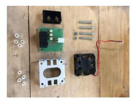
7 Put the head PCB back together. Start with inserting the four bolts through the new head PCB:
