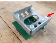
11 Slide the fan on the four bolts with the red-black cable protruding from the same side as the opening in the fan guard. Also fasten the two hex nuts (on the right side for the left extruder, and vice versa):
