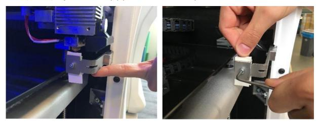
Note ; the Bolt has one silicon wiper per extruder where the Bold Pro has two silicon wipers per extruder. On the Bolt Pro the silicon wipers should all be calibrated at the same height.
