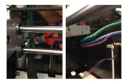
Using a flat-head screwdriver, open the second to last shackle of the drag chain to loosen it from the last (fixed) shackle. Also, loosen the second to last shackle in the back of the machine, so the whole drag chain is loose:
