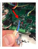
11 Unplug the two small white connectors on the left side of the electronics board with the thin white and green cables going into them:
