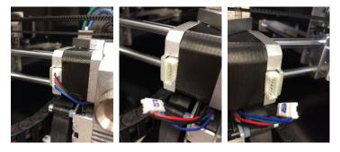
4 Move the motor cable and plug to the side of the extruder head, and then pull through the bearing and cooling block:
