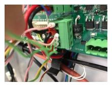
31 Connect the **single brown** and **grey wires** into the big wide green connector. The two brown wires go together in the leftmost slot, the grey wires go together in the second slot (as seen from the left):
