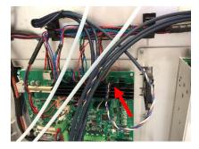
26 Then connect the right motor cable to the EMOT2 connector on the electronics board:
