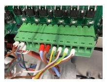
34 The wiring is now done (see end result below), and the back cover can be placed back using the six 3mm bolts.
