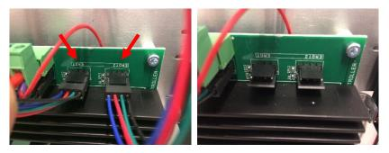
Unplug the two black square connectors in the middle of the electronics board. These connectors have white and orange cables going into them. Loosen the retainer plug of the connector and then gently pull them back:
