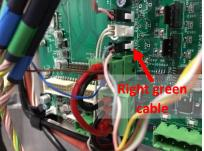
29 Connect the black four-pin connector into the left square black connector on the electronics board. Connect the same connector from the right cable on the right black connector:
