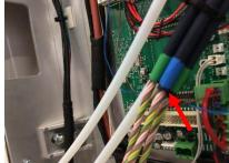
28 Connect the black two-pin thermistor from the left green cable into the top thermistor slot. Connect the black two-pin connector from the right green cable into the bottom thermistor slot:
