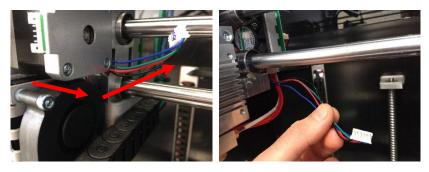
Cut the tie-wraps on the side of the extruder which hold all the cables:
