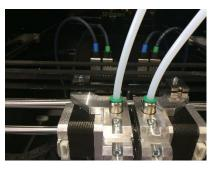
19 Take the new motor cable (white-black-brown-blue) with the white connector, and put it from the top in between the top bearing and rear cooling fan. Then, guide it over the bottom bearing, and through the side of the extruder (i.e. to the left in the left extruder). Then, guide it in between the radial cooling fan and the extruder motor to the front. Finally connect it to the extruder motor. Do this for both extruders:
