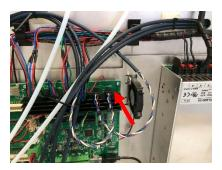
Using two tie-wraps, fix the four remaining cables to one of the white filament tubes. Don't tighten the tie-wraps too much (they will stay in place due to friction with the mantle of the cable). Make sure the ends of the cables line up:
