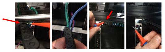
Repeat for both drag chains, then move to the back of the machine. Unplug the two rightmost motor connectors (labelled EMOT and EMOT2):
