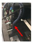
Only for the left extruder: apply a tie-wrap on the left RJ45 connectors in order to pull the cables closer to the extruder head (i.e. pull the cable against the blue RJ45 connector). Make sure when sliding the left extruder all the way to the left, that the cables are not touching the left side of the carriage with the X-motors:
