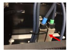
o the back of the printer. Apply tie-wraps to the cables in order to fix them to the
