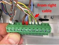
33 Connect the big green connector carefully back into the electronics board:
