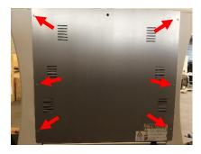
2 After removing the back plate, unplug the green and blue cables from **both the extruder**s heads:
