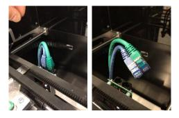
Unplug the white 6-pin connector from **both** the left and right extruder motors:
