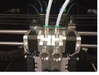
20 For both extruders, apply tie-wraps to the cables and the aluminium strut at the bottom of the extruders:
